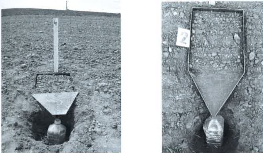
Fig. 1 A microplot for surface runoff collection installed after the crop sowing, a collector directing water runoff to a collection bottle is covered with a sheet metal
