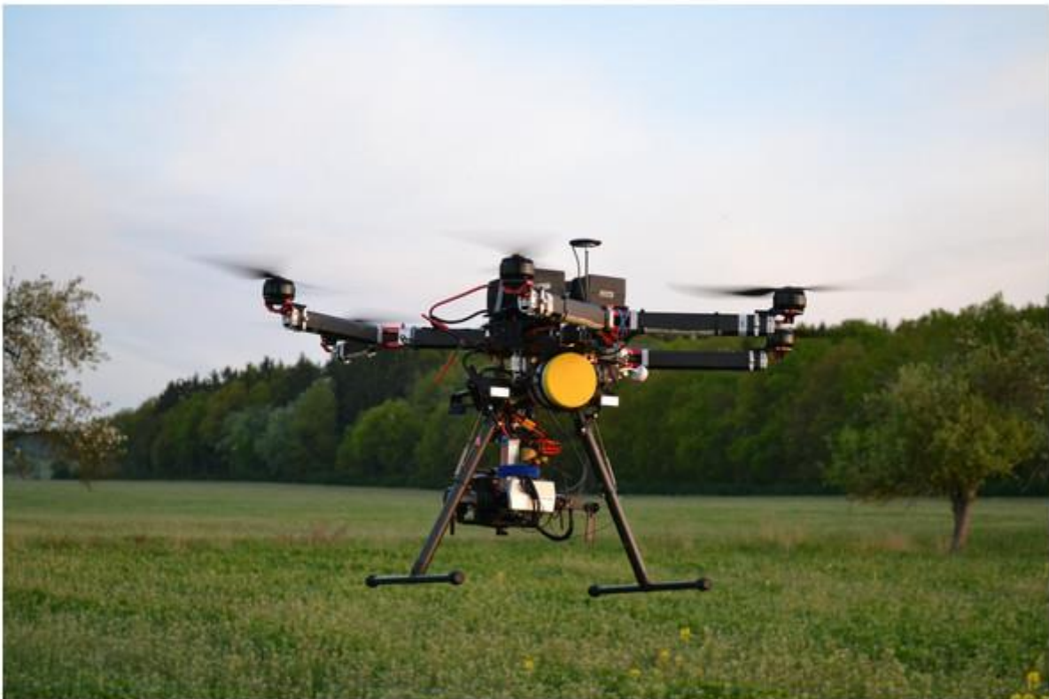
Figure 7: HEXACOPTER GD HX-1100F ZODIAC UAV equipped with a Workswell WIRIW 2nd gen. camera.
