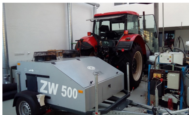
Fig. 1 Dynamometer MAHA ZW 500, connected to the tractor Zetor Forterra 8641
