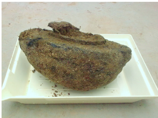
Fig. 3. The cake that is formed at the input of liquid cattle manure from the chamber No. 6 (Fig. 1) to the chamber No. 7 (Fig. 1), has the shape of a mushroom turned upside down and corresponds to the supposed seepage path of liquid cattle manure through the subsoil
