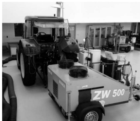
Figure 1. The tractor Zetor 8641 with mobile dynamometer MAHA ZW 500.
