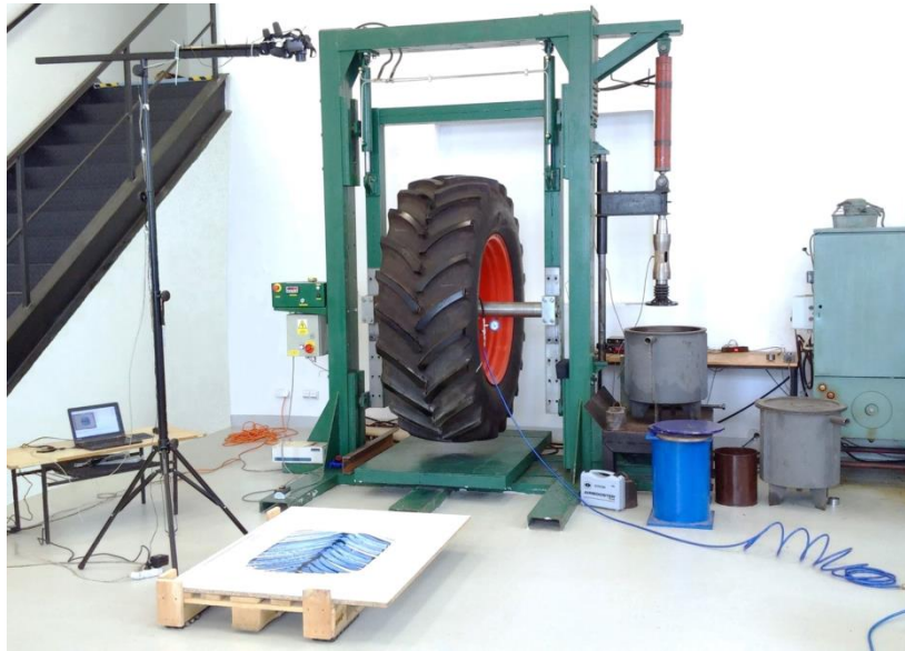
Fig. 1. Testing of traction tire Mitas 650/65 R 38 (RD-03) and laboratory equipment.
