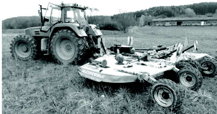
Figure 2. Working set – tractor Fendt 818 with connected Mulcher MZ 6000.
