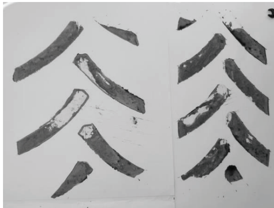
Figure 3. Tyre footprints – left MITAS AC 85, right – MITAS VF (load 4.29 kN).
