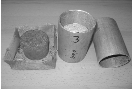
Fig. 1. Briquette in a metal basket ready for “unlimited water sorption” (left), briquette in a tube ready for “limited water sorption” (right)
