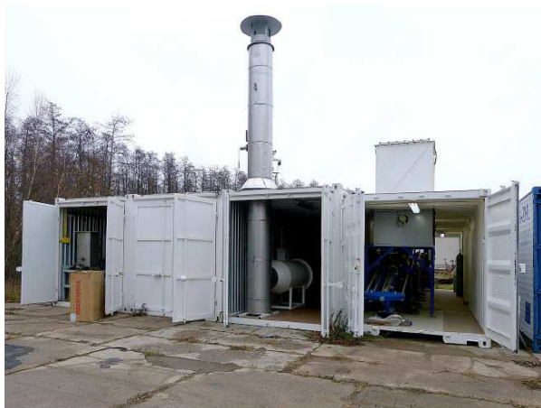
Fig. 15: Container placing of development and testing technological line VÚZT, v.v.i. Prague - PolyComp, a.s. Poděbrady for carbonization and gasification of residues and waste with performance of 20 kg/h input feedstock
