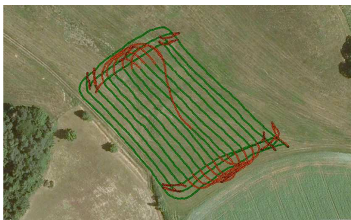
Fig. 22: Trajectory of tractor set with mulcher during the continuous mulching of plot
