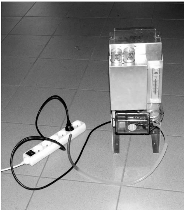
Fig. 4. Ozone measuring equipment APOA 350 E in the diagnostic vehicle
