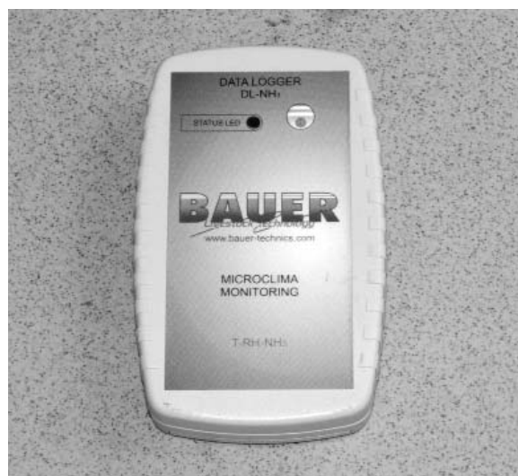
Fig. 2. Measuring equipment for confirmation of reaction O 3 -NH 3
