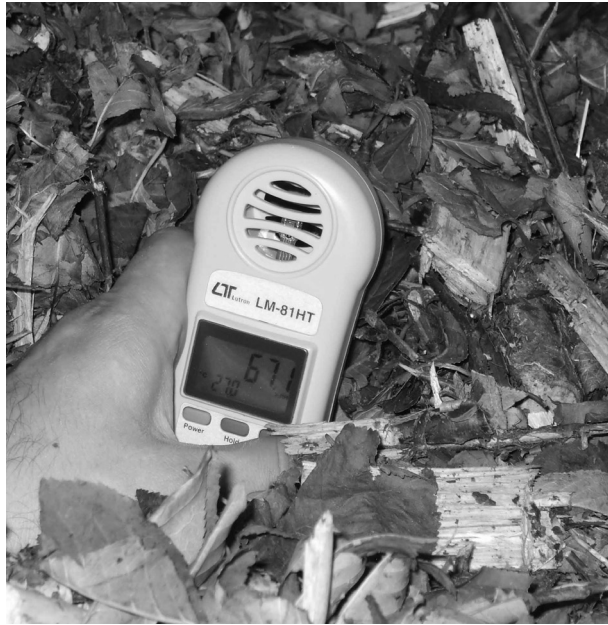
Fig. 6. Electronic psychrometer Lutron LM-81HT
