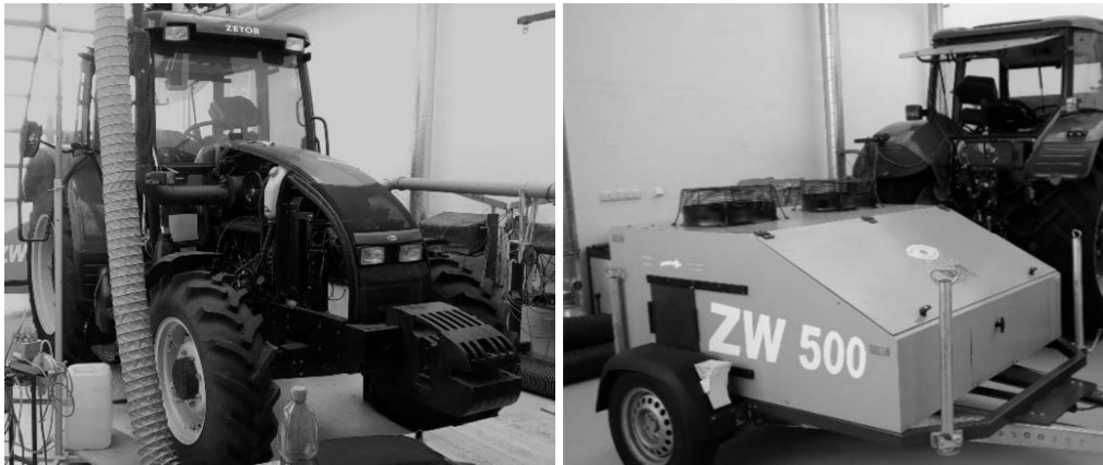
Figure 1. Tractor Zetor 8641, used for measurement (left), mobile dynamometer MAHA ZW 500 (right).
