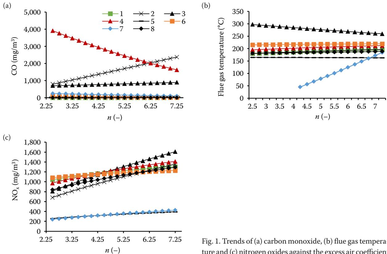
Fig. 1. Trends of (a) carbon monoxide, (b) flue gas temperature and (c) nitrogen oxides against the excess air coefficient
